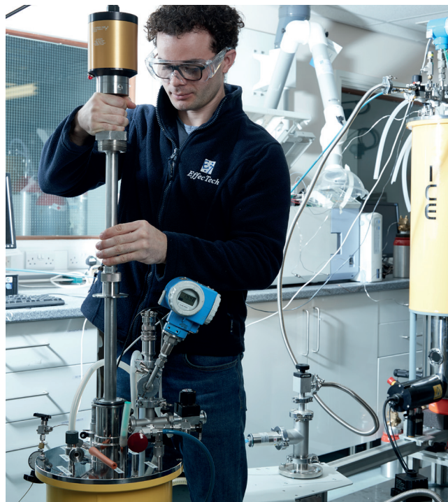
Dr Joey Walker inserting the LNG probe into the custom-built EffectTech liquefier
